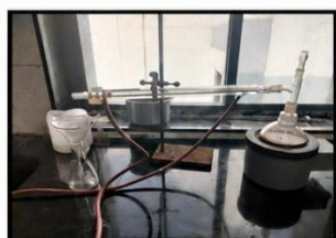
Fig 1 (e) Preparation of Shirishadi Arka by distillation apparatus
